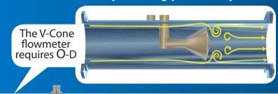
The V-Cone flowmeter acts as its own flow conditioner by disrupting all centralized flow disturbances.
