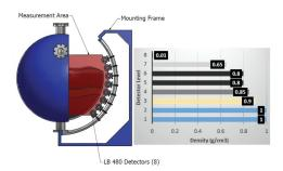
The Multiphase Level System measures the density profile in the separation tank
