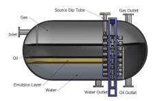
Arrangement of Multiphase Level Measurement on an oil separator with a rod source and several detectors mounted outside
